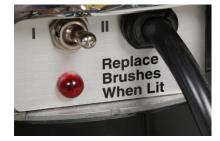
The dual speed model has a simple switch to change from 180 to 320 rpm. Also, there is an indicator light that illuminates when the carbon motor brushes need replacement.
