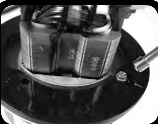
8. Remove remaining 3 screws which attach compression ring to motor.
