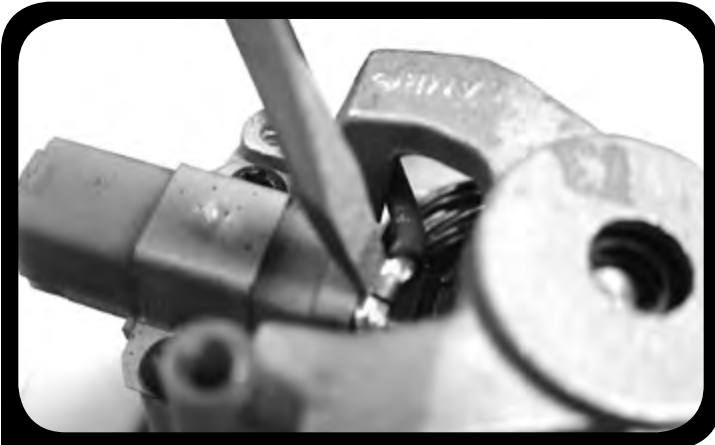
6a. Use end of flathead screwdriver, gently wedge between center of motor brush and clip. Turn screwdriver counter-clockwise to push out the wire clip under the motor brush insulation.
