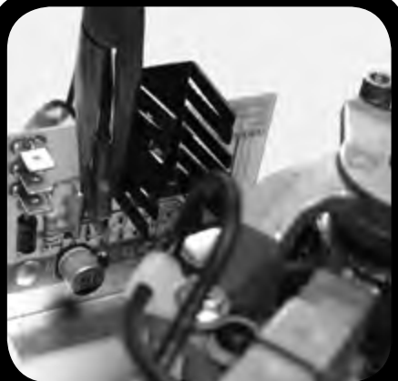
6. Remove thermal switch connector from BCM.
