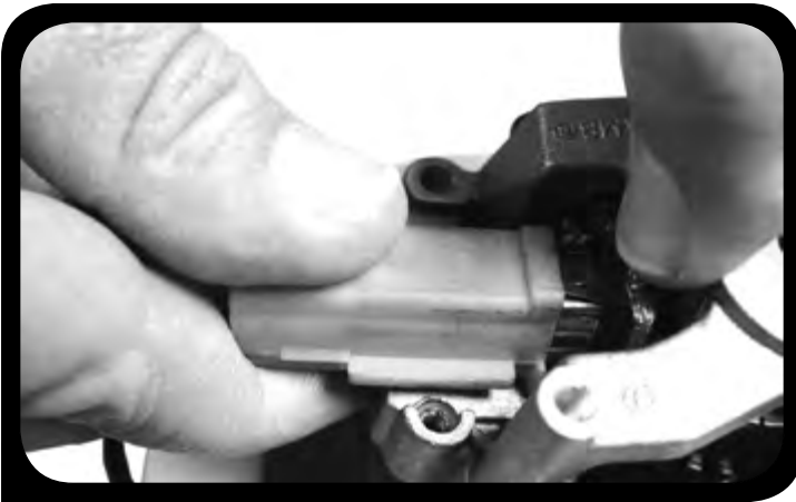
8. Remove motor brush. Remove 2nd motor brush in same way. Tip brush upward and slide connector out.
