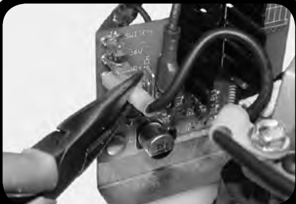
5. Remove horizontal motor connector from BCM.
