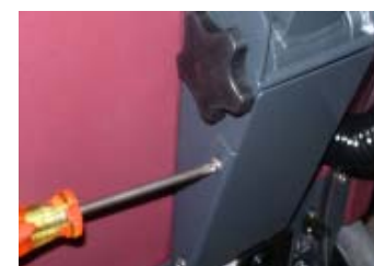
Screw the cover back with the 4 screws.
