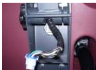
Attach the wire harness to the machine.
