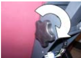
Spin the adjustment knob clockwise to tighten.
