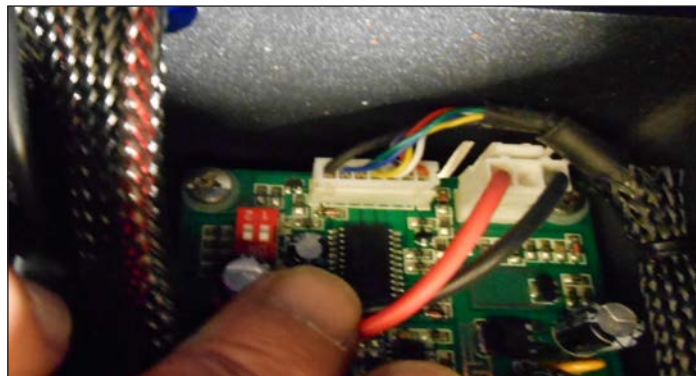
Figure 4. Showing the Communication cable connector at the Control PCB
