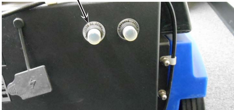
Vacuum Motor circuit breaker
