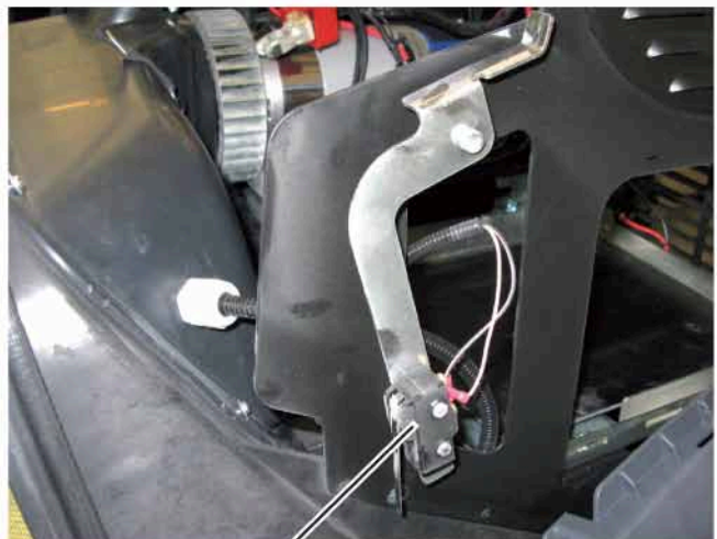
Hopper position microswitch (SW0)
