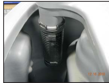
Tank Float Shutoff
