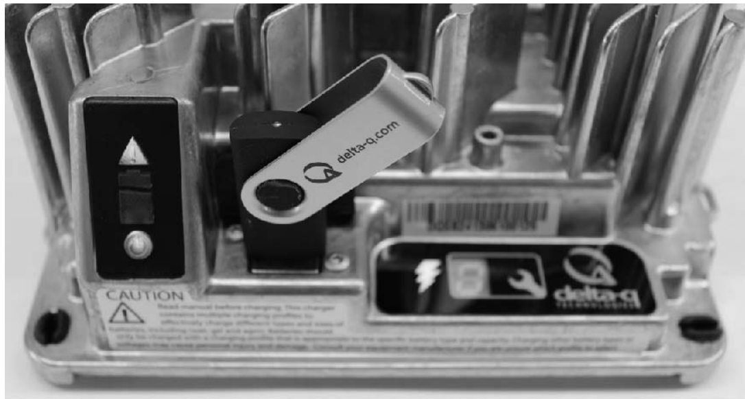
Figure 5, Insert the USB flash drive to begin the charge data download process. This step can be completed using the same USB flash drive programmed to update the charger's software. The process is completed when the USB indicator is solid green, and no longer flashing.
