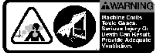
TOXIC GASES LABEL - LOCATED ON THE CONTROL PANEL
