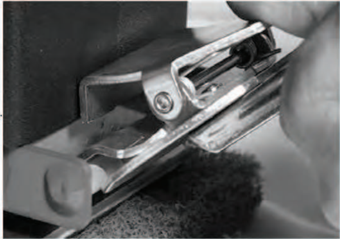
***figure 3 Correct way of attaching handle to the Doodle Scrub base.
