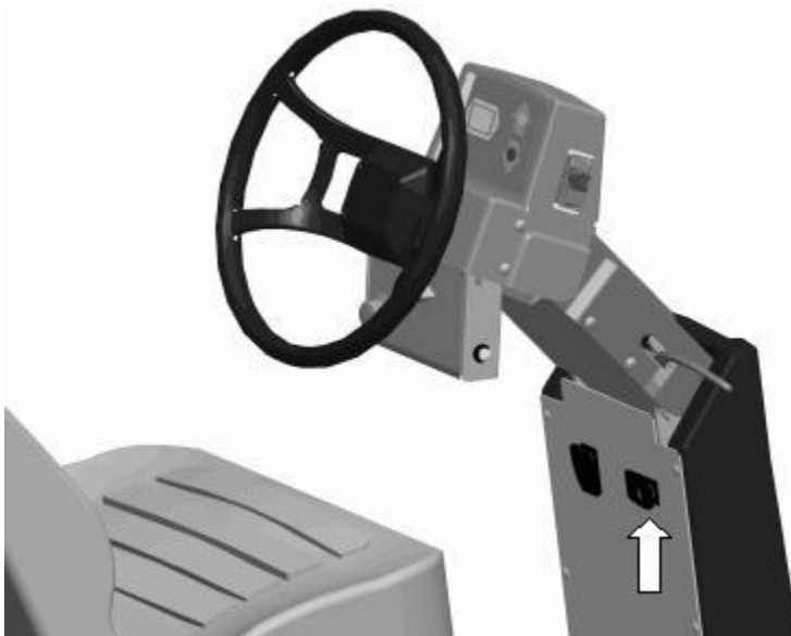
Location of Side Shift Switch
