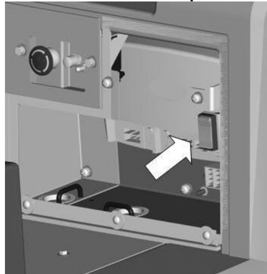
Manual Override Switch, located behind electrical panel.
