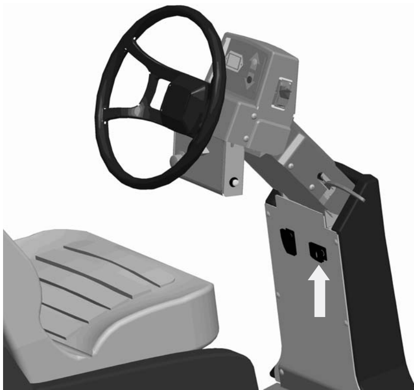
Location of Side Shift Switch
