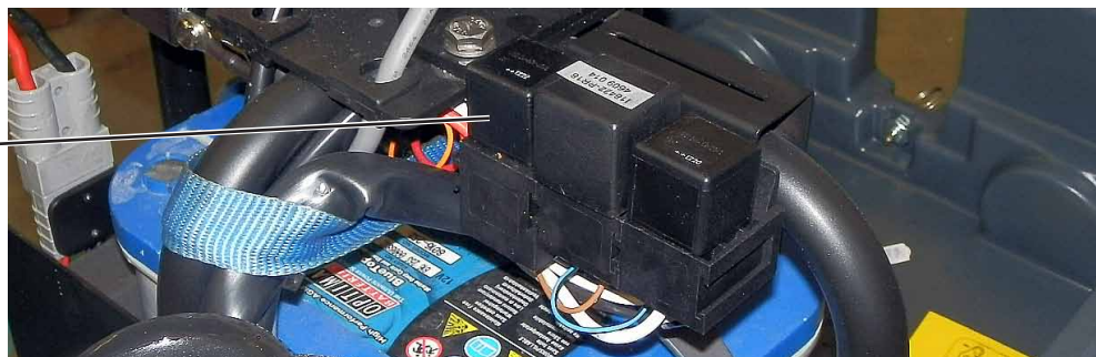
Brush motor relay (K1)
