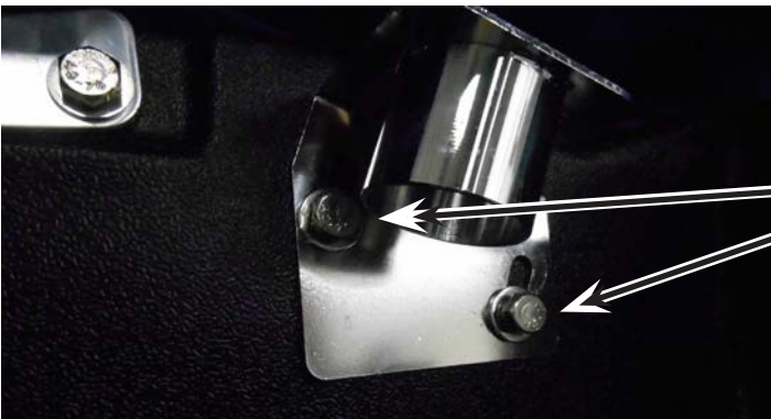
Bolts for adjusting pick-up tube adapter bracket
