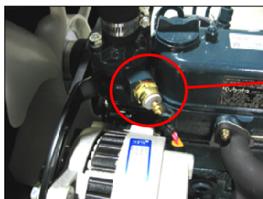
Coolant Temperature Sensor (above alternator)
