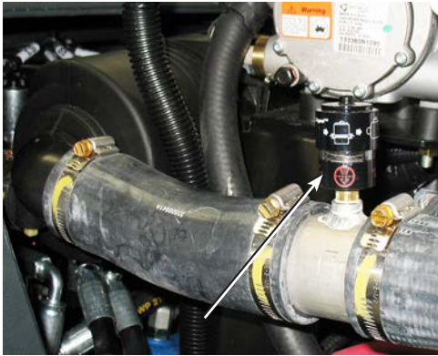
Air Mechanical Vacuum Filter Service Indicator Location
