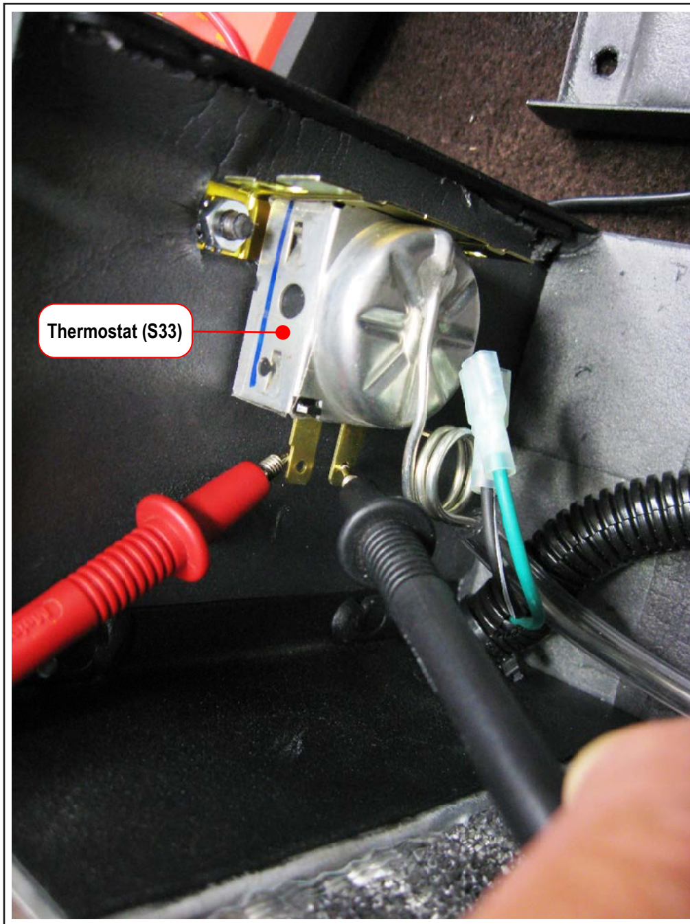
Figure 11. Checking Continuity through the Thermostat
