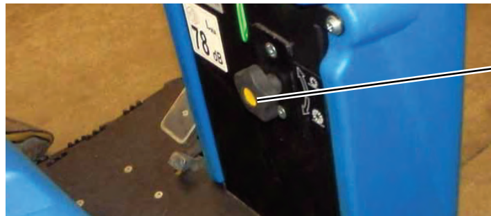
Main broom height adjusting knob
