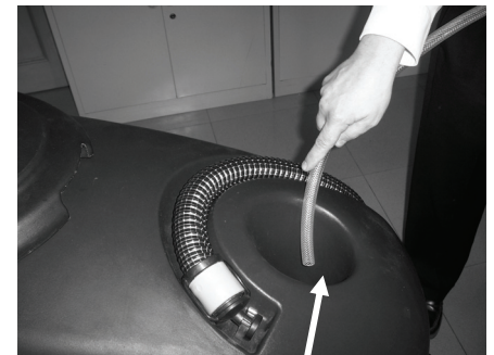
Solution Tank Fill Opening
