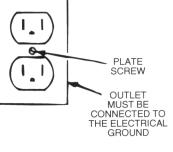
This machine uses a 120 volt AC 60 cycle electrical circuit. Make sure you have the correct frequency and voltage before connecting the power cord to an outlet. The machine has a plug as shown in Figure 1. If a receptacle connected to the electrical ground as shown in Figure 1 is not available, have one installed by an electrical contractor. Do not use an adapter.
