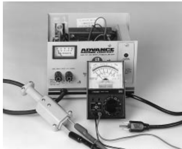
FIGURE 8. Test charger DC circuit. The circuit does not conduct in reverse direction.
